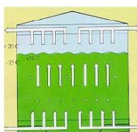
In a composter, air conditioning is done using the difference between the temperature inside the compost and outdoor temperature,
