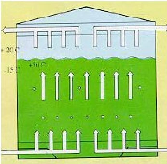
In a composter, air conditioning is done using the difference between the temperature inside the compost and outdoor temperature,
